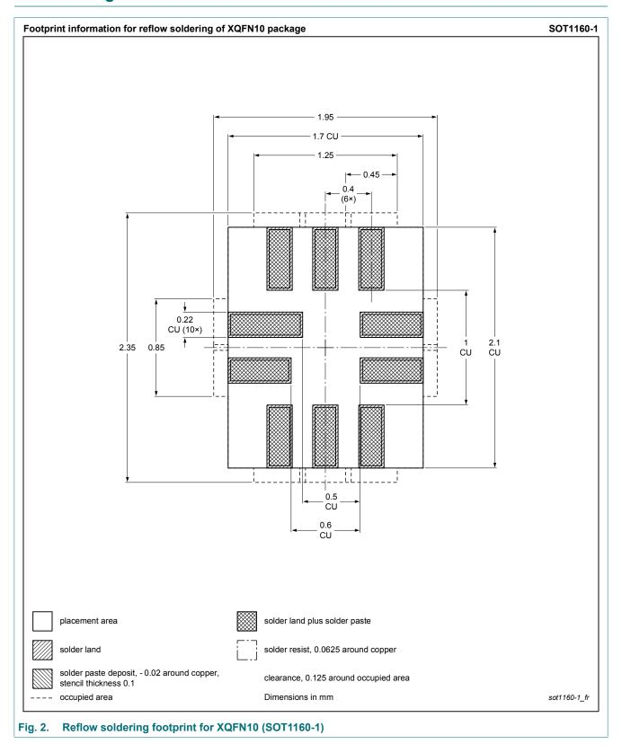
plastic, leadless extremely thin quad flat package; 10 terminals; 0.4 mm pitch; 1.4 mm x 1.8 mm x 0.5 mm body
